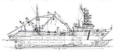
The catch disgorged from the seine net can be sent directly below decks to one of seven separate refrigerated holds that have a combined capacity of 669m<sup>3</sup>. Unusually for a fishing vessel of this type, the holds take up the whole aft end of the vessel with the engine room located forward beneath the superstructure.
